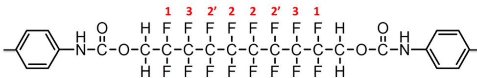
Figure 6. Structure of the biodegradable fluorine-containing polyurethanes.
