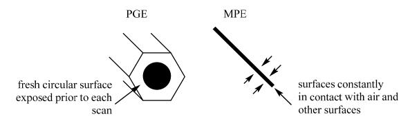
Figure 5. Diagram of PGE vs. MPE, highlighting the difference in exposed surface area.
