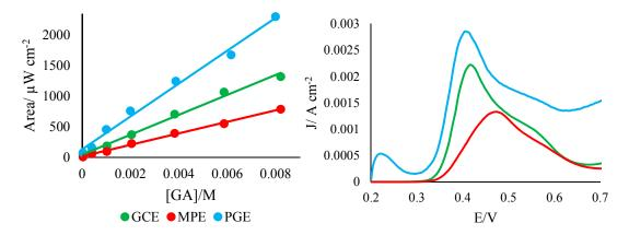
**Figure 2.** Characterization of PGEs in gallic acid standards. Left: calibration curves for electrodes in gallic acid ([GA] =  $8 \times 10^{-3}$ - $4 \times 10^{-5}$  M, n = 4); Right: representative voltammograms of electrodes in gallic acid ( $2 \times 10^{-3}$  M). To account for differences in exposed area, current is given as a function of raw current divided by electrode surface area.
