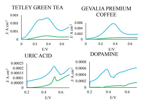
**Figure 4.** Proof of principle. Representative voltammograms of the PGEs (blue) and GCEs (green) in samples of coffee, tea, UA (0.00001 M) and DA (0.00001 M). To account for differences in exposed area, current is given as a function of raw current divided by electrode surface area.
