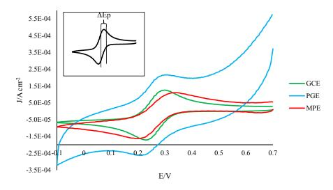
**Figure 1.** Representative voltammograms of GCE, MPE and PGE electrodes in 1 mM ferricyanide solution. To account for differences in exposed area, current is given as a function of raw current divided by electrode surface area. Initial potential = 0.7 V; vertex potential = -0.1 V; final potential = 0.7 V; scan rate = 0.05 V/s.
