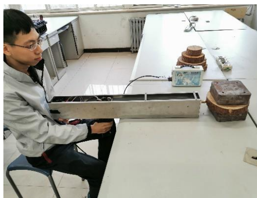
Figure 11. The operation of the microdestructive tree-ring measurement system.
