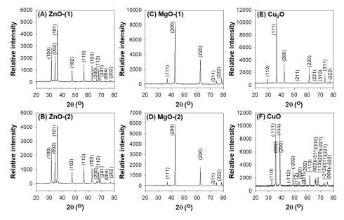
**Figure 2.** PXRD patterns of metal oxide (MO) particles: (**A**) ZnO-(1), (**B**) ZnO-(2), (**C**) MgO-(1), (**D**) MgO-(2), (**E**) Cu<sub>2</sub>O, and (**F**) CuO.
