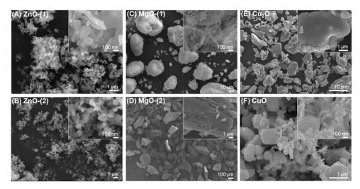
**Figure 1.** FE-SEM images of metal oxide (MO) particles: (**A**) ZnO-(1), (**B**) ZnO-(2), (**C**) MgO-(1), (**D**) MgO-(2), (**E**) Cu<sub>2</sub>O, and (**F**) CuO.
