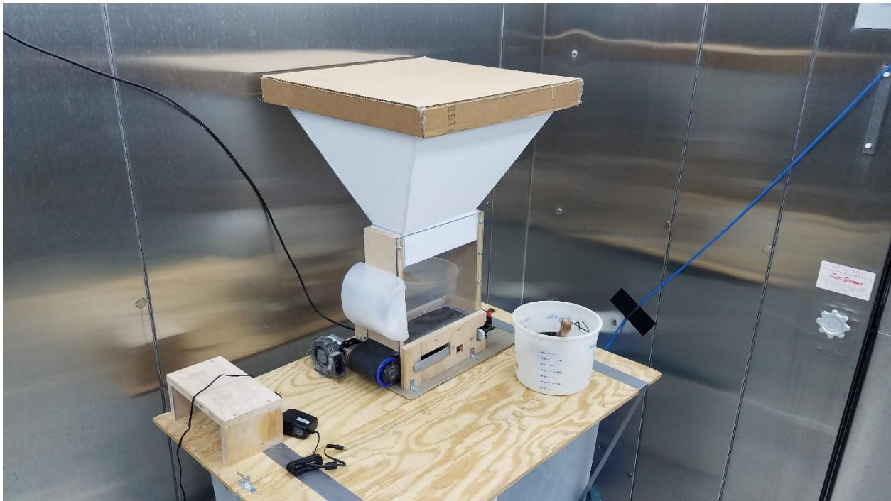
Figure 12. Dust generator placed in controlled environment chamber.
