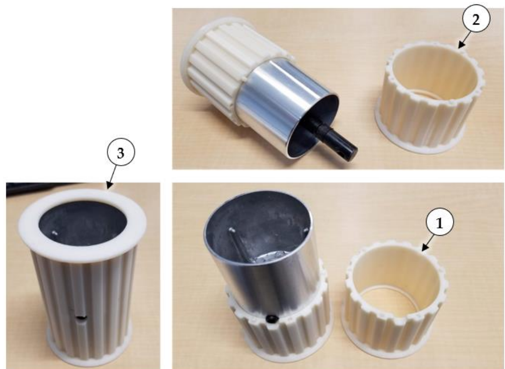
Figure 4. Split mating halves of 3D printed (1) drive and (2) idler pulleys, and (3) drive pulley halves assembled and glued onto aluminum drive pulley.
