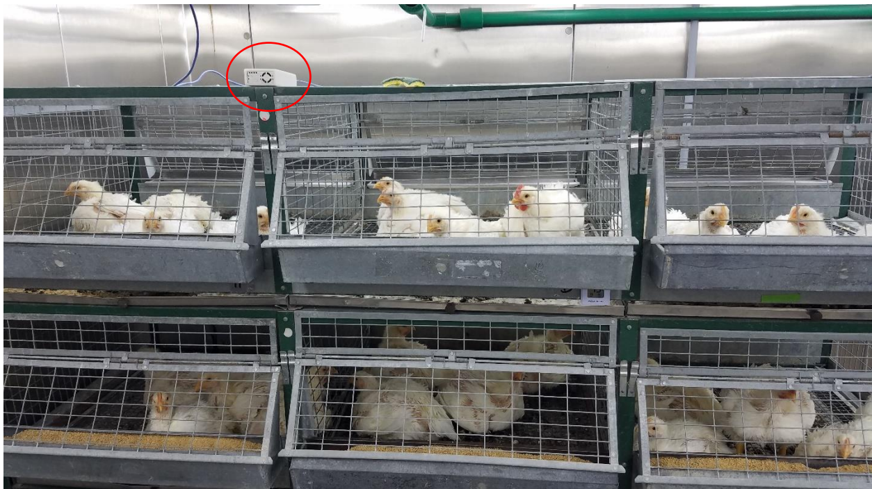
Figure 13. PMS5003 dust sensor enclosure (circled in red) placed on top of laying hen cages.
