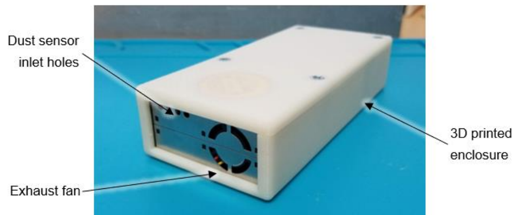
Figure 1. PMS5003 dust sensor mounted in 3D printed enclosure.
