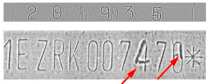
Fig. 6. Using magneto-optical imaging to examine stamped markings in metal substrates. (a) Magneto-optical image of manipulated digits on one of our test-panels: “3” (second left) was sanded out and restamped with “0”. “6” (4. left) was cut out, the cut segment turned by 180° and re-inserted to make it a “9”. “4” (far right) was stamped over to make it a “5”. (b) Magneto-optical image of manipulated digits in an original vehicle identification number (see red darts): “6” (far right) was changed to “8”. “1” (4. right) was restamped to make it look like “4”. (For interpretation of the references to color in this figure legend, the reader is referred to the Web version of this article.)
