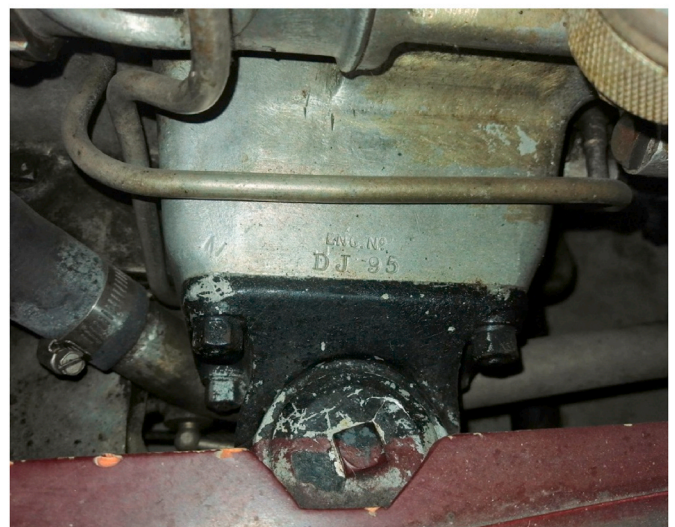
Fig. 2. Numbers stamped on technical components that can identify a vehicle. (a) Original chassis number on a 1938 Lancia Aprilia. (b) Original engine number on a 1933 Rolls-Royce Phantom II.
