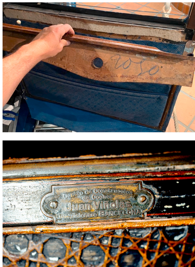
Fig. 8. Historical markings can help to clarify the local and chronological context of elements and materials preserved on a vehicle. (a) Body number 2090 of a 1931 Delage D8L, applied by the upholsterer during the production process with blue wax crayon on the back of a wooden interior trim panel. Such markings, both how they were applied, and their location can give clues to the manufacturer of the body, its upholstery and interior trim, as well as to their initial affiliation with the vehicle in question. (b) A coach builder’s plaque on a 1900 Renault type C, relating to body modifications commissioned by the first owner located in Spain. (For interpretation of the references to color in this figure legend, the reader is referred to the Web version of this article.)
