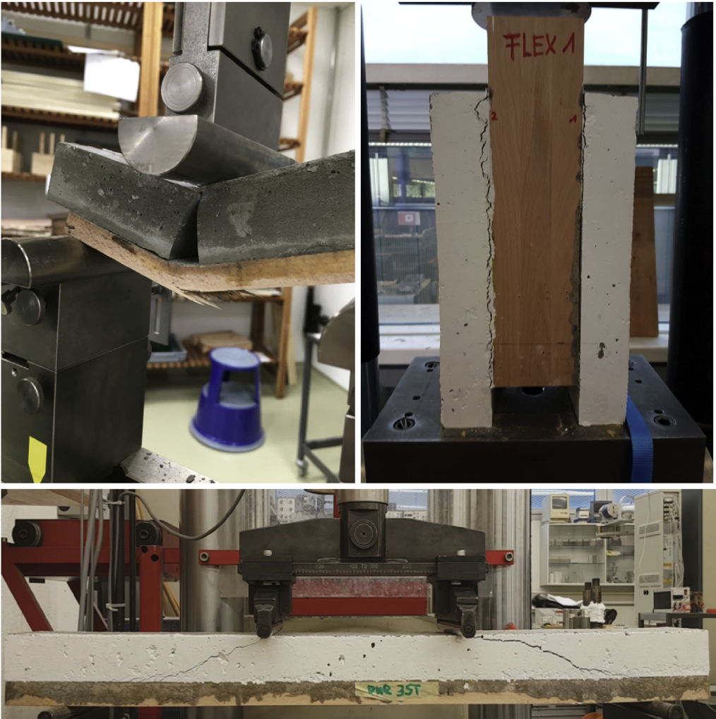
Fig. 3. Setups of all three loading conditions after the failure of the composites. The image on the upper left side shows the 3-point-bending test; the image on the upper right side shows the push-out test, with the described ‘sandwich’ geometry of the specimen and at the bottom is the 4-point-bending test. All pictures show the cracked specimen in order to illustrate the failure behaviour.
