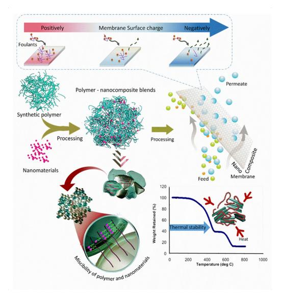
**Figure 9.** Illustration of the preparation of a PPSU nanocomposite membrane with higher surface and thermomechanical properties via a typical polymer and nanomaterial blend system.
