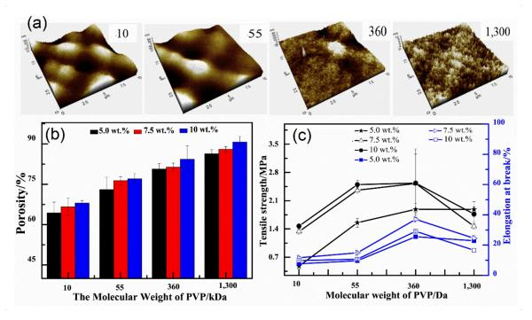
**Figure 8.** PPSU UF membranes with different molecular weight of PVP: (**a**) AFM images; (**b**) porosity; (**c**) tensile strength.
