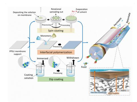
**Figure 11.** A schematic of the PPSU surface modifications using physical and chemical surface modification techniques.
