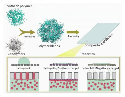
**Figure 6.** Schematic illustration of the preparation of PPSU membrane with superior properties via a typical polymer and copolymer blend system.
