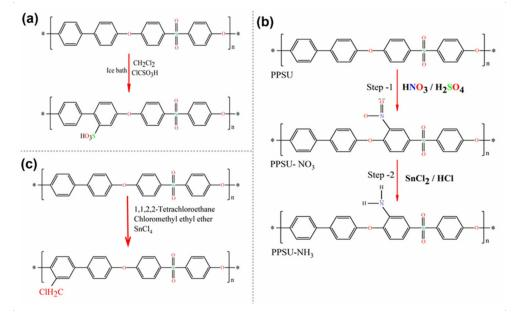
**Figure 4.** Synthesis of polyphenylsulfone. Reaction pathways: (**a**) sulfonation; (**b**) amination; (**c**) chloromethylation.
