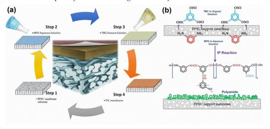
**Figure 14.** PPSU membrane surface modification schematic diagram: (**a**) steps in the modification process; (**b**) interfacial polymerization reaction mechanisms during the formation of the TFC layer.
