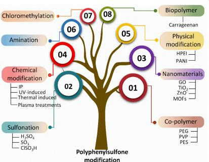
chloromethylation; (2) blending with a synthetic polymer, inorganic nanomaterials, and biopolymer; and (3) surface modification via physical and chemical approaches (Figure 2).
