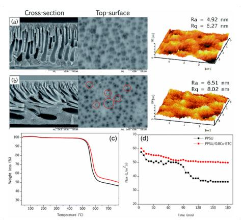
**Figure 10.** PPSU membranes embedded with Cu-BTC; SEM images of cross-section, top surface and 3D AFM images: (a) PPSU; (b) PPSU/Cu-BTC; (c) TGA curves; (d) flux profile membranes.
