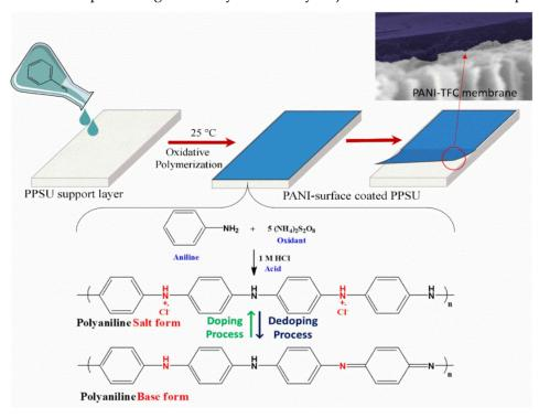
**Figure 12.** PANI-surface Polyphenylsulfone membrane surface coating via the chemical oxidation of monomeric aniline.
