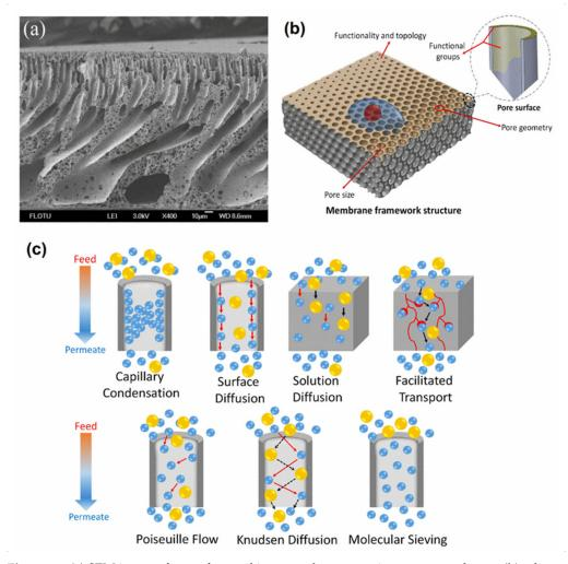
**Figure 13.** (a) SEM image of manufactured integrated asymmetric porous membrane; (b) schematic representation of pore size, pore geometry, pore surface, and structure of porous polymers; (c) schematic illustration of foremost transport mechanisms.
