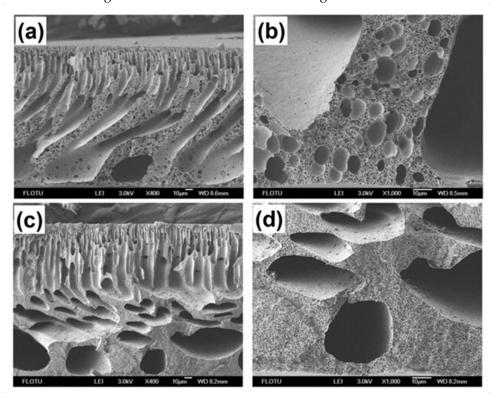
**Figure 7.** SEM photomicrographs of cross-sections of PPSU UF membranes prepared with: (**a**,**b**) PVP-15000; (**c**,**d**) PEG-6000 as a polymeric pore-forming additives.
