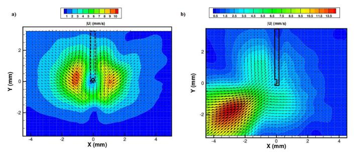
**Figure 5.** Time-averaged maps of velocity magnitude and velocity vectors. The needle is located along the axis x = 0 (for y > 0) and the port is centered in the point x = (0, 0), the position of the cutter is sketched on each map. (a) Front view, (b) lateral view with the cutter port on the negative side of the *x*-axis. Twenty-five gauge, TDC, core mode, and 4000 cpm.
