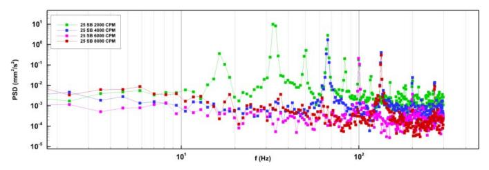
Figure 6. Power spectra of the kinetic energy per unit mass. Each curve corresponds to a different cutter. SB front view. Pressure = 600 mm Hg.
