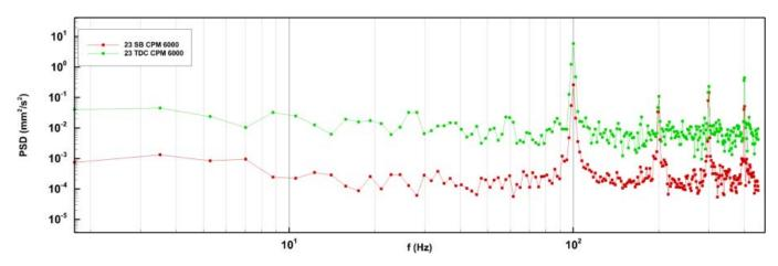
Figure 3. Power spectra of the fluid kinetic energy per unit mass. Experiments with BSS, pressure = 600 mm Hg, cpm 6000.
