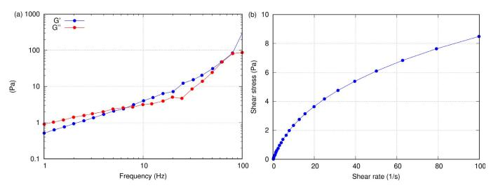
**Figure 1.** (a) Storage *G*' and loss *G*'' moduli versus the oscillation frequency f (1–100 Hz). Strain  $\gamma = 0.05$ . (b) Shear stress  $\tau$  versus shear rate  $\gamma$ . Temperature, T = 23°C. Note that the dependency of the complex modulus on the strain is relatively small, lower than 10%. Measurements at 37°C are not shown, owing to the relatively small dependence of the moduli on temperature, of the order of 40% for *G*' and less than 20% for *G*''.
