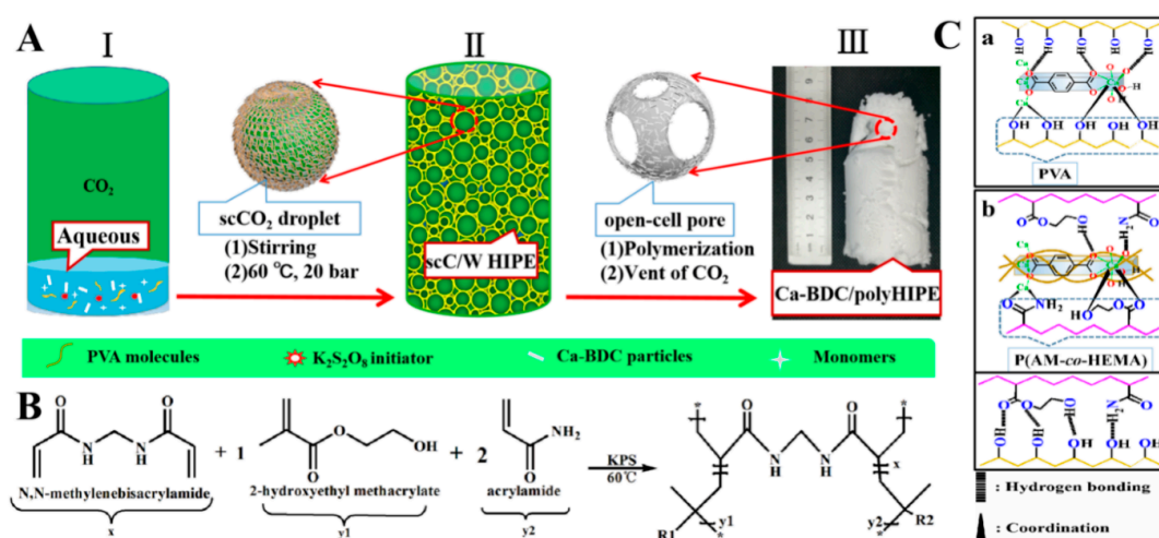
Scheme 1. (A) Schematic illustration for the preparation of Ca-BDC/P(AM-co-HEMA)HIPEs; (B) typical radical polymerization of 2-hydroxyethyl methacrylate (HEMA), acrylamide (AM), and N,N -methylenebisacrylamide (MBA) initiated by potassium persulfate (KPS) ( x = n wt %, y_1 + y_2 = 100 - n wt %) at 60 °C; (C) interactions between individual components in Ca-BDC/P(AM-co-HEMA) HIPEs.
