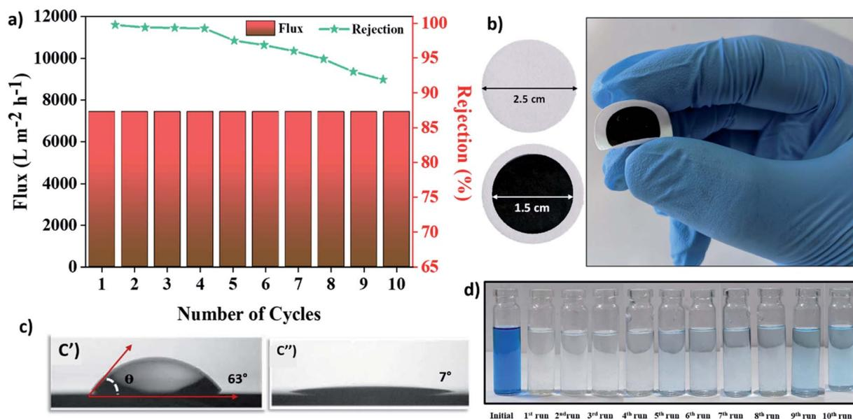
Fig. 6 (a) Regeneration study of Mn<sub>3</sub>O<sub>4</sub>/AHC for adsorption of MB dye. (b) Photograph of Mn<sub>3</sub>O<sub>4</sub>/AHC powder-based membrane. (c) Contact angle measurements for the prepared membranes. (c') AHC membrane, (c'') Mn<sub>3</sub>O<sub>4</sub>/AHC membrane. (d) Digital photograph of permeates obtained during the recyclability study.
