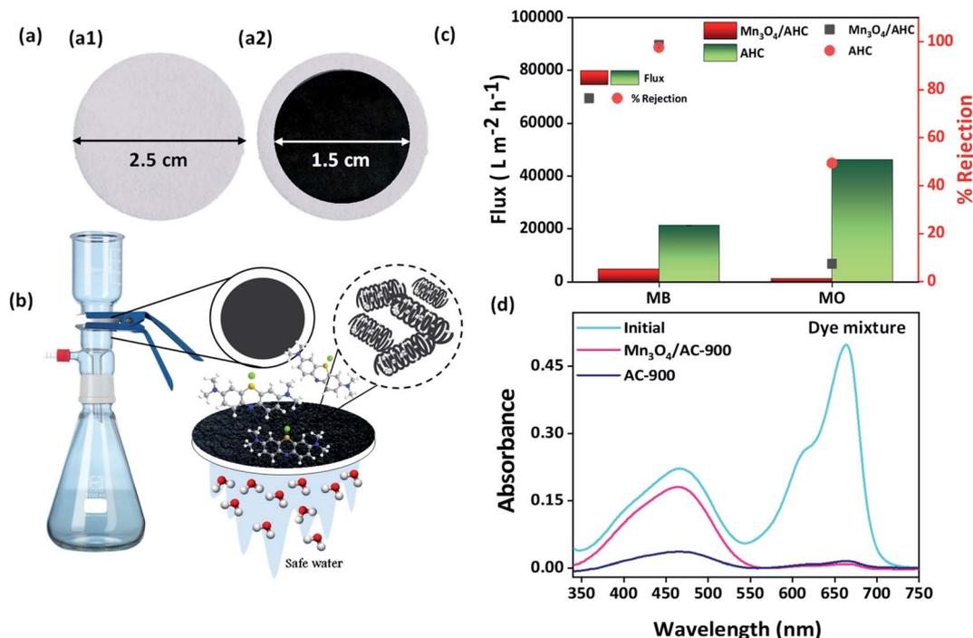
Fig. 4 Photographs of (a1) Whatman filter paper (a2) filter paper after  $\text{Mn}_3\text{O}_4/\text{AHC}$  via vacuum filtration. (b) Lab-scale continuous flow filtration setup for organic contaminant removal. (c) Flux and rejection for AHC and  $\text{Mn}_3\text{O}_4/\text{AHC}$  for MB and MO dyes removal via continuous flow and (d) UV-Vis spectra for dye mixture (MB + MO) removal using the prepared materials.
