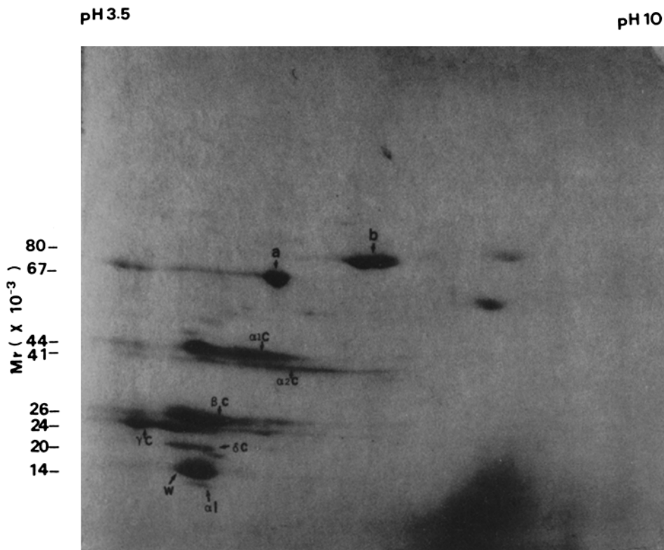
FIGURE 1 Two-dimensional gel electrophoresis of mouse skim milk. 300 \mu g of milk protein was precipitated with trichloroacetic acid, washed with acetone, and dissolved in lysis buffer containing 9.5 M urea, 2.0% NP-40, 5% \beta -mercaptoethanol, 1.6% pH 5-7, 0.4% pH 3.5-10 ampholine. First dimension was nonequilibrium pH gradient electrophoresis with acidic end on left and basic end on right. Second dimension was SDS 6-15% PAGE. The gel was stained with Coomassie Blue to visualize the spots. a, albumin; \alpha_1c , \alpha_2c , \beta c , \gamma c , and \delta c , \alpha_1 -casein, \alpha_2 -casein, \beta -casein, \gamma -casein, and \delta -casein, respectively; W, whey acidic protein; al, \alpha -lactalbumin; b, an 80,000-mol-wt protein, most probably transferrin.
