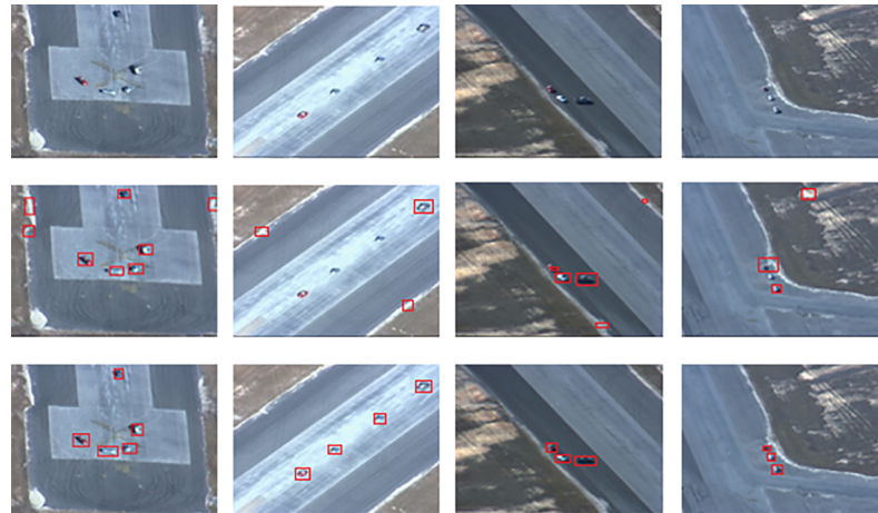
Fig 9. Visual comparison for moving target detection methods. The first row is original images, the second row is frame difference method and third row is our proposed method.
