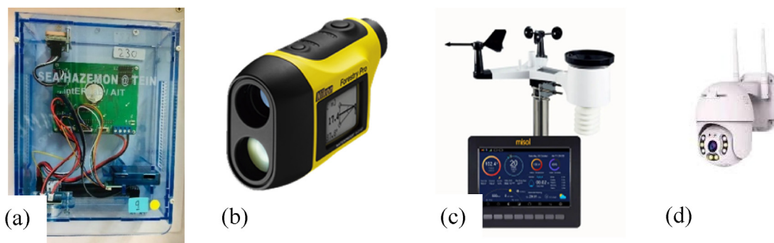
Figure 4. Equipment used for the study (a) SEA-HAZEMON PM 2.5 sensor, (b)Nikon Forestry Pro I, (c) Microclimate sensor and display and (d) CCTV camera.
