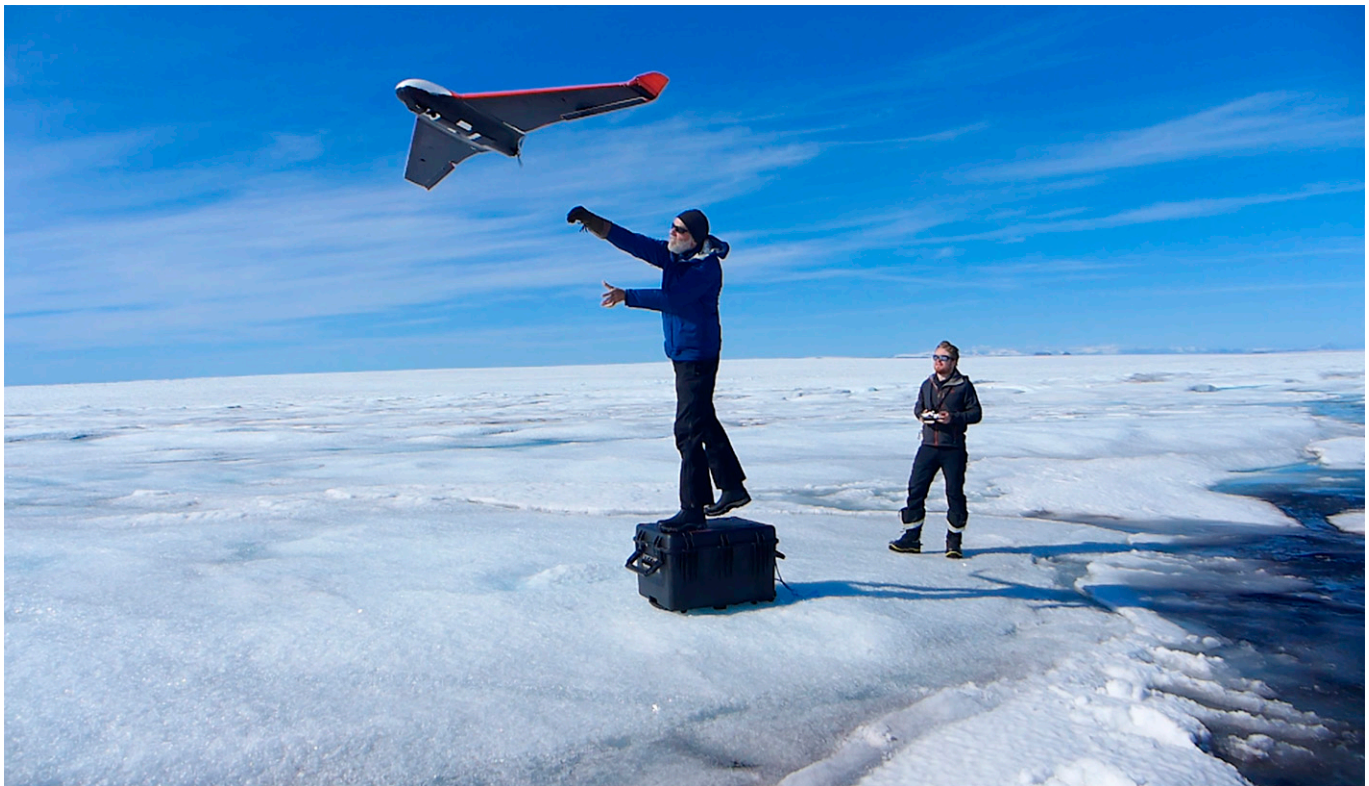
Unmanned aerial vehicles (UAVs) are among the tools that researchers use to monitor drainage from the meltwater lakes that sit atop ice sheets. Image credit: Tom Chudley.
