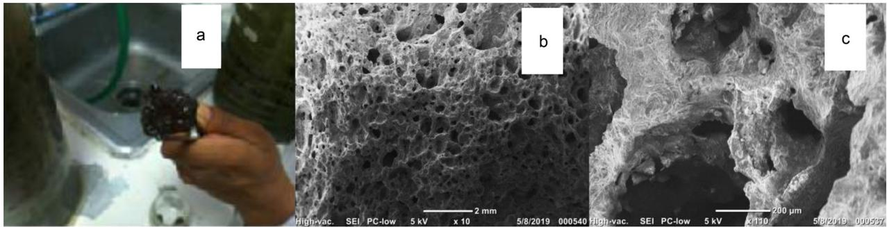
Fig. 6. Properties of tezontle as supporting material of the SBR. a) A piece of tezontle containing adhered peritrichous colonies; b) Scanning Electron Microscopy (SEM) of tezontle stones; c) closeup of tezontle pores.
