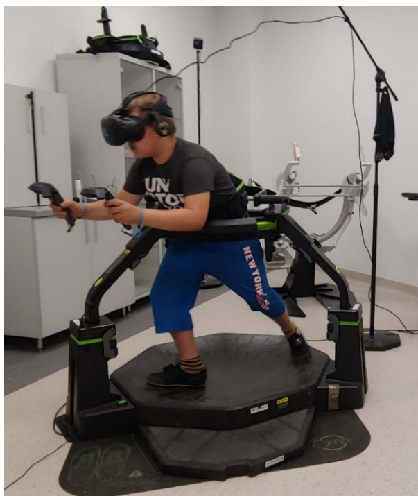
Figure 1. Test stand: participant on an OMNI omnidirectional treadmill playing an active video game (AVG) in immersive virtual reality (IVR).
