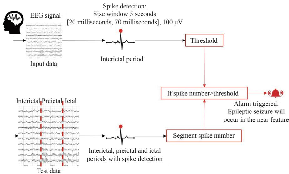
**Fig. 3 Diagram of the proposed seizure prediction method.** The spike number obtained from the interictal period will first be used as a threshold. The segment spike number in the preictal period is then compared to this threshold and the alarm will be triggered when it exceeds it.
