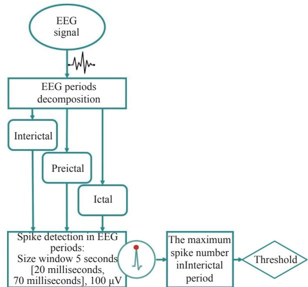
**Fig. 1** Block diagram of EEG spike detection method.
