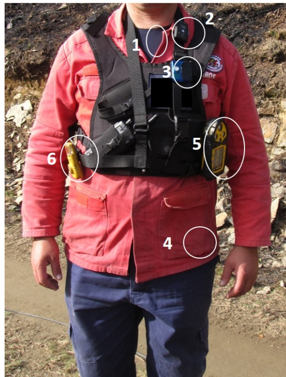
Figure 1. VR2 equipment: (1) VitalJacket ® t-shirt; (2) GPS; (3) FREMU; (4) Smartphone; (5) GasAlert Extreme CO; (6) GasAlertMicro 5 PID.
