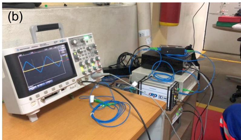
Figure 9. (a) Point in the engine where the FBG pressure sensor was installed and (b) interrogator and the demodulator tool kit installed in a control room 50 m from the engine under test.
