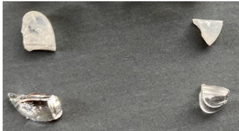
Figure 1. Photo-image of (100 - x) (33\text{CaO-67B}_2\text{O}_3) - x \text{Ca}_3\text{WO}_6 ( x = 4 (Left) and 8 (Right)) glass before (Downward) and after (Upward) heat-treatment.
