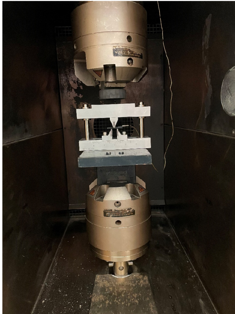
Figure 1. Test Setup showing Short Beam Shear Test Setup with AE sensor inside the environmental chamber.
