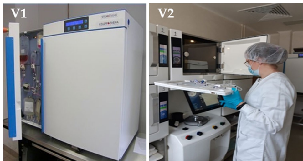
Fig. 1 The StemXpand® cell expansion platform: V1 clinical version with one incubator and production kit (left); and the V2 clinical version (on process) comprising 5 incubators and an aseptic cassette replacing the previous kit of production (right)
