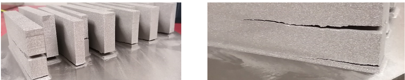
Figure 4. Destructiveness of residual stress due to the temperature gradient [76] (Courtesy of CRPM).
