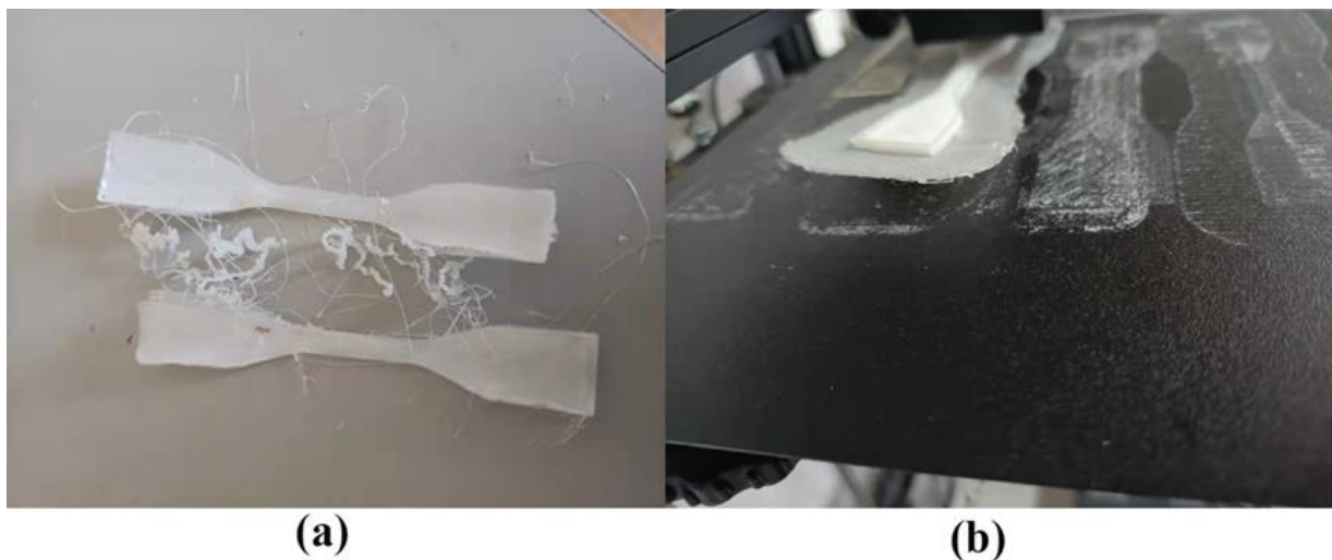
Figure 7. (a) Failed print while taking 7 parameters; (b) wrapped print at 245 °C.
