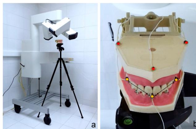
**Figure 2.** (a) Articulo-graph, tripod, and mouth anatomical model configuration; (b) placement of sensors on the mouth anatomical model (active sensors, yellow; reference sensors, red).
