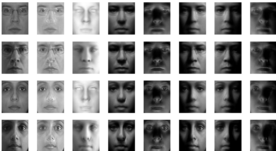
Figure 6. Relit images based on the Multi-PIE database (1st column: input image; 2nd: recovered texture; 3rd: estimated illuminance; and 4–8th: relit images).
