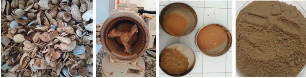
FIGURE 1: The followed steps in the preparation of adsorbent powder from almond shells: almond shells' grinding, sieving, and size grading. Almond shell powder (ASP) for adsorption essays.
