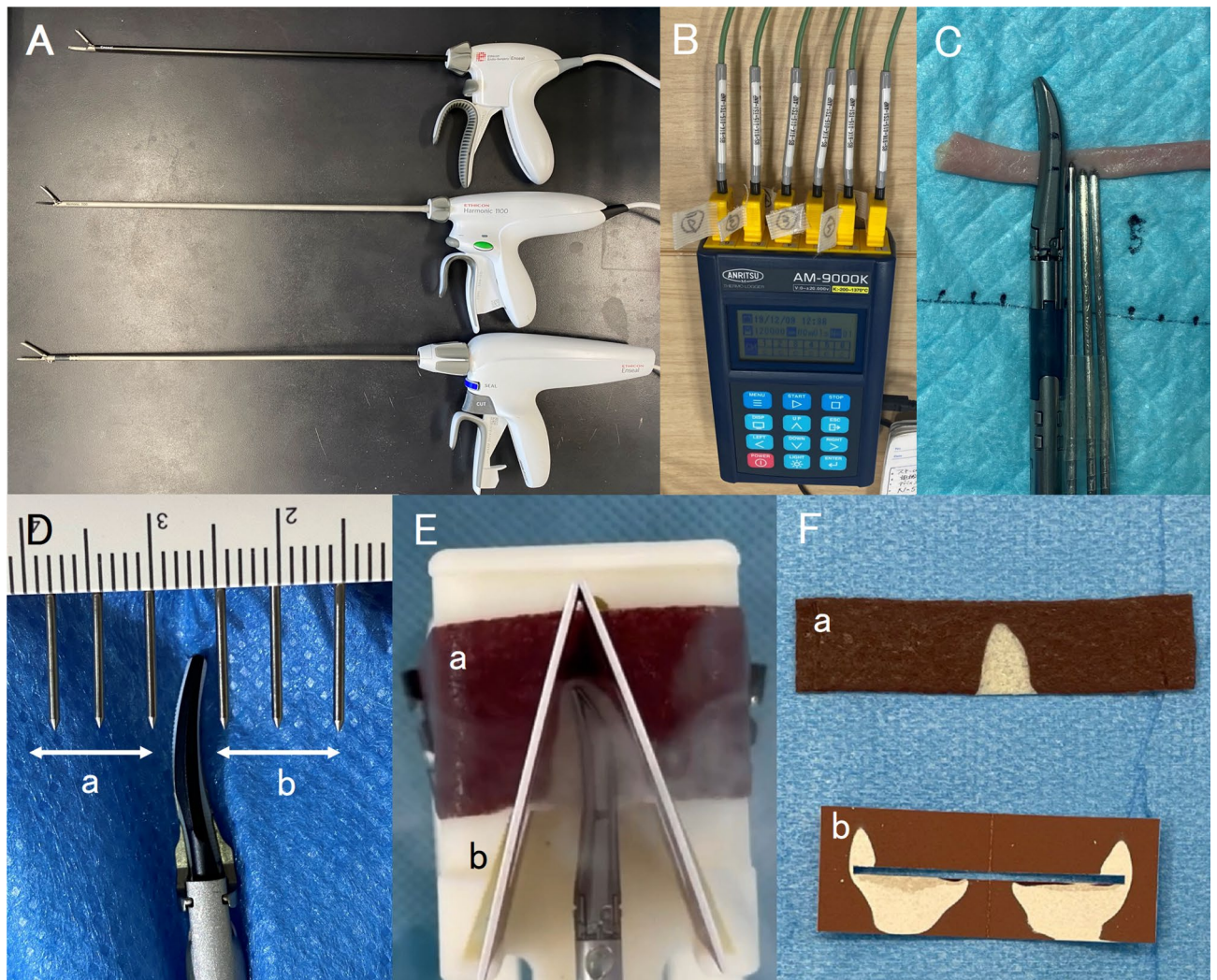
Fig. 1. (A) Energy devices employed in this study: ENSEAL™ G2 Curved Tissue Sealer, HARMONIC® HD1000i Shears, and ENSEAL™ X1 Curved Jaw Tissue Sealer (from top to bottom). (B) Six-channel model of AM-9000 K thermocouple. (C) An ex-vivo model analyzing the direct thermal effect. A pin electrode was placed into the tissue, and the temperature was recorded at 1, 3, and 5 mm away from the energy device. (D) An ex-vivo model analyzing the indirect steam thermal effect. A pin electrode was placed above the jaw grasping tissue, and the temperature of the surrounding space was recorded at six different points from the grasping site (1, 5, and 10 mm of the outside (a) and inside (b)). (E) An ex-vivo model analyzing the steam thermal spread of energy devices. Versatile Training Tissue (VTT), whose color changes from brown to white at approximately 50 °C, was located horizontally (a) and vertically (b). The center of the VTT was grasped and activated once an energy device was used. (F) VTT after activation of energy device (a: horizontal sheet, b: vertical sheet). The steam spread area was calculated by the sum of the white areas of both horizontal and vertical sheets.
