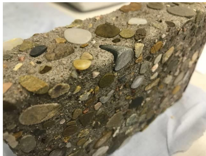
Figure 9. Corroded concrete prism of SCC-Slag after seven months of exposure to sulfuric acid of pH 2.
