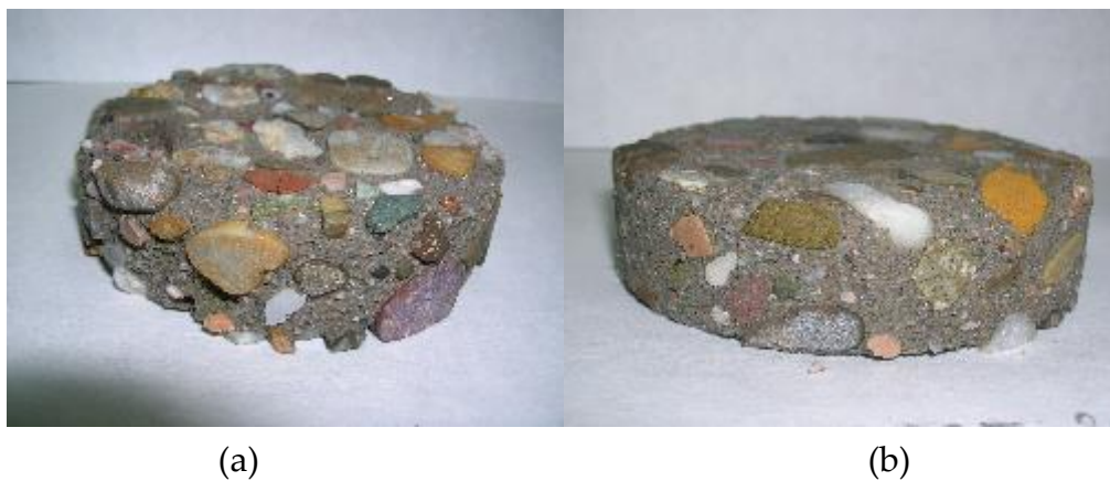
Figure 15. The corroded concrete slices after 3 months in H_2SO_4 at pH 2–4: (a) SCC-Slag concrete samples brushed; (b) sonicated.
