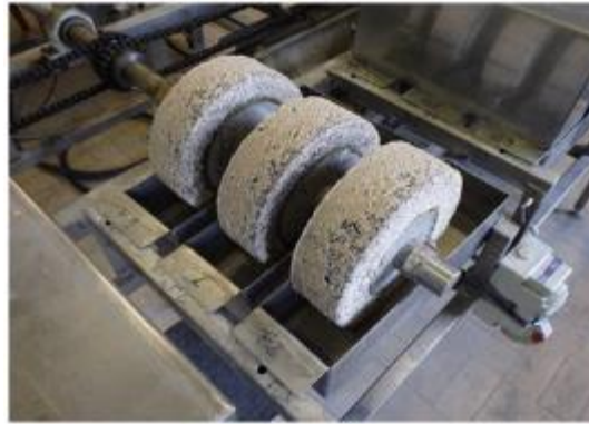
Figure 5. Example of concrete degradation with the accelerated TAP method.
