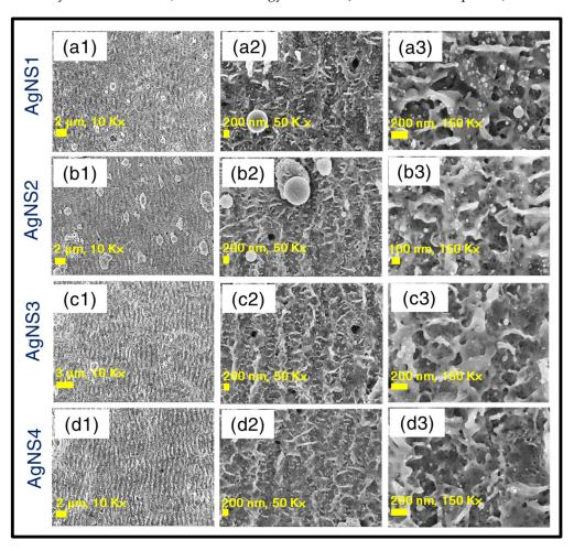
**Figure 3.** FESEM images for AgNS1 ((**a1–a3**)-12 mJ), AgNS2 ((**b1–b3**)-16 mJ), AgNS3 ((**c1–c3**)-20 mJ), AgNS4 ((**d1–d3**)-24 mJ), respectively. For the four sets of images for each NS, in detail, all figures corresponding to labels (1), (2), (3) illustrate FESEM images with different magnifications of  $10~{\rm K}\times$ ,  $50~{\rm K}\times$ ,  $100~{\rm K}\times$ , respectively.
