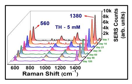
**Figure 13.** Stability data of the 20 nm Au-coated AgNS2 in sensing TH (5  $\mu$ M) molecule, illustrating a superior performance compared to bare AgNS2.
