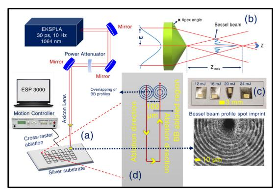
**Figure 1.** (a) Schematic of the experiment involving BB ablation in the air on Ag. The cross-raster scanning employed is also depicted in the figure with BB profile imprint observed at the initial ablation spot (indicated by the dashed line and inset), (b) Axicon prism lens and the generated BB, (c) pictures of the fabricated silver NSs with different input pulse energies (12 mJ, 16 mJ, 20 mJ, and 24 mJ), (d) Schematic of overlapping two BB profiles during the first raster scan.
