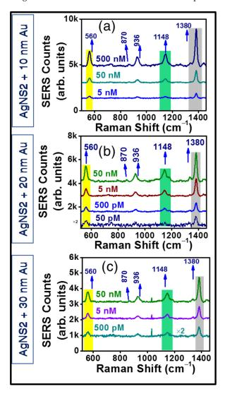
**Figure 10.** Concentration dependent SERS spectra of Au coated AgNS2 substrates in the detection of TH molecule. The lowest trace limits have been exhibited to be 5 nM from 10 nm coating (**a**), 50 pM from 20 nm coating (**b**), and 500 pM from 30 nm Au deposition (**c**). The best trace detection efficiency was achieved with 20 nm Au coated AgNS2.
