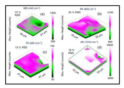
**Figure 8.** SERS mapping data of AgNS2 obtained with a micro-Raman spectrometer engaging 25% (of full power) of 532 nm laser, a  $50\times$  objective, with the following experimental parameters: acquisition time 5 s, accumulation number 3 and a mapping step size of  $10~\mu m$ . A 3D representation of the Raman-mapped area of ~(45  $\mu m \times 50~\mu m$ ), probing various molecules as (a) MB, (b) PA, (c) TH, (d) AN is presented.
