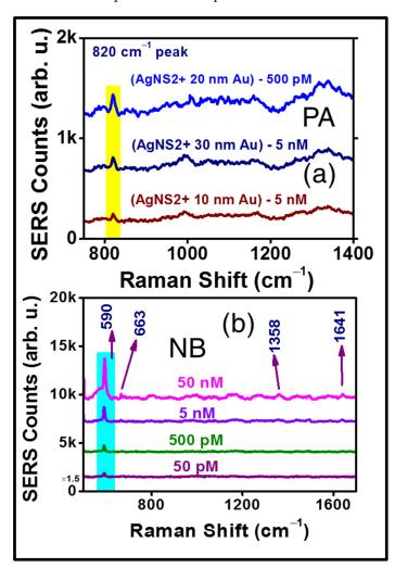
**Figure 11.** (a) SERS spectra of PA molecule, confirming the lowest trace detection was 500 pM with (AgNS2 + 20 nm Au) substrate (b) concentration dependent SERS spectra of NB, with 50 pM lowest trace being detected.
