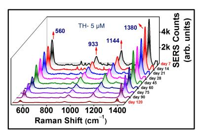
**Figure 9.** Stability data of AgNS2 while sensing TH (5  $\mu$ M), illustrating the significant 560 cm<sup>-1</sup> peak along with others. The SERS data were collected up to 120 days.
