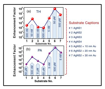
**Figure 6.** Enhancement factor comparison from the sensing performances of (a) TH (b) PA. These studies involved all the Ag NSs along with different thickness of Au coated AgNSs. Lowest detection limits (displayed in light blue colour) and enhancement factors (displayed as solid symbols; lines are only a guide to the eye) of each substrate are presented. '#' refers to the sample number.
