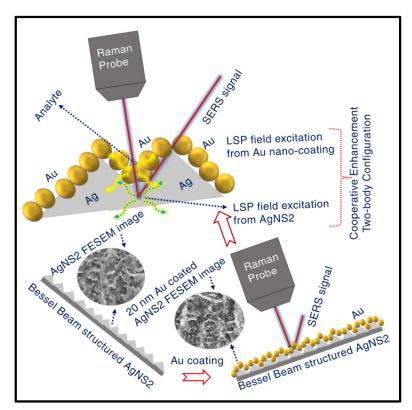
**Figure 12.** Schematic of Au coated AgNS2 explaining the mechanisms giving rise to cooperative enhancement from two-body system (AgNS2 + 20 nm Au). An evanescent electric field excitation is demonstrated in two-body system due to an appropriate match in penetration-depth condition.
