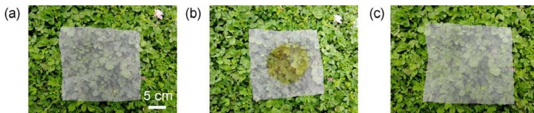
**Figure S10.** Photographs of Ag-nylon electrode as PM filter, Related to Figure 4. (a) as-fabricated, (b) after PM filtration and (c) after cleaning process.
