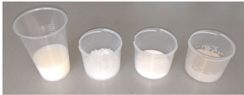
Figure 3. Accelerators involved in the research, from left: crystal seeds admixture, calcium nitrate, sodium hydroxide, CKD.
