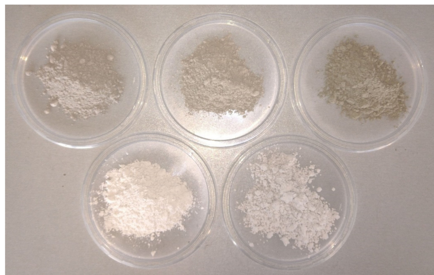
Figure 2. Clinkers (top row, from left C1, C2, C3), GGBFS (bottom row left), and anhydrite (bottom row right) involved in the research.
