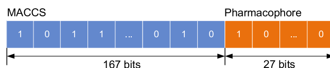
Figure 2. Fragment feature representation, splicing the 167-bit MACCS fingerprint with the 27-bit pharmacophore feature.
