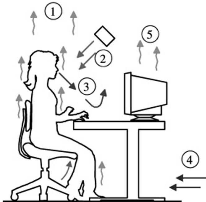
**Figure 10.** Interaction between airflows generated by various sources around the human body in an office environment: (1) free convective flow, (2) personalized flow, (3) respiratory flow, (4) ventilation flow, and (5) thermal flow (reprinted with copyright permission from [102]).
