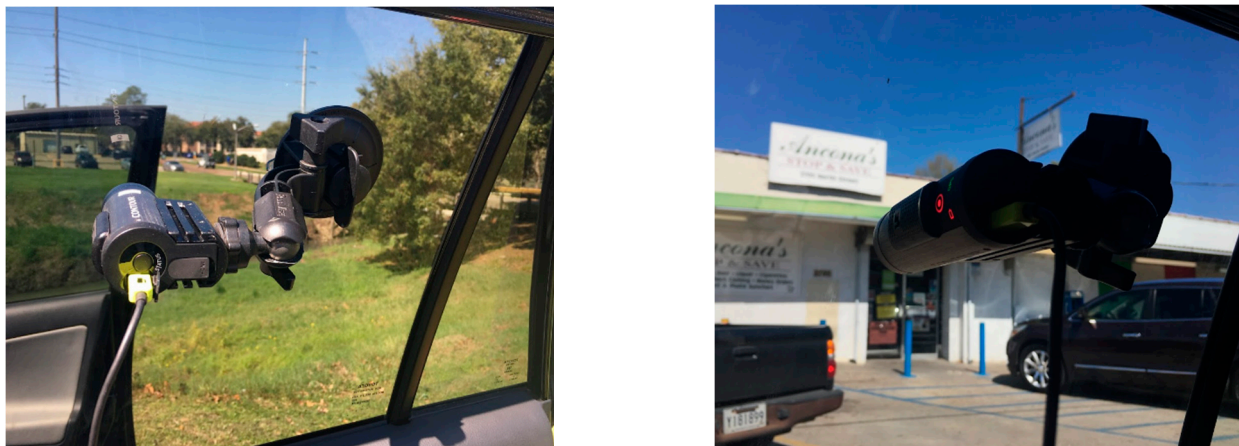
Figure 2. Examples of spatial video cameras mounted to the inside window of a vehicle.
