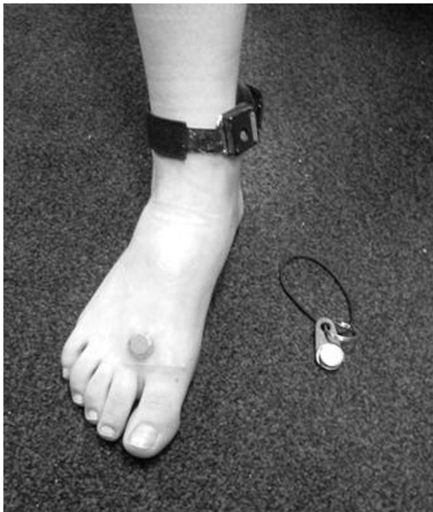
Figure 1 —Setup for measuring ambulatory foot temperature. One iButton is attached to the foot; the other is attached to a key ring apparatus that can be affixed to external clothing. The actigraphy monitor is attached to the ankle as well.
