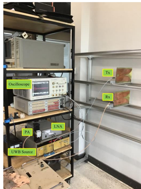
Figure 8. Experimental setup of the through-wall UWB radar.
