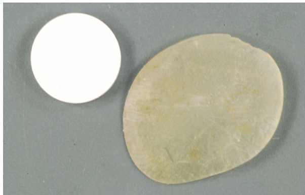
Fig. 2. Ivory cross-section 1 cm in diameter and 300 \mu\text{m} thick next to a calcium phosphate pellet used to calibrate the photographs.
