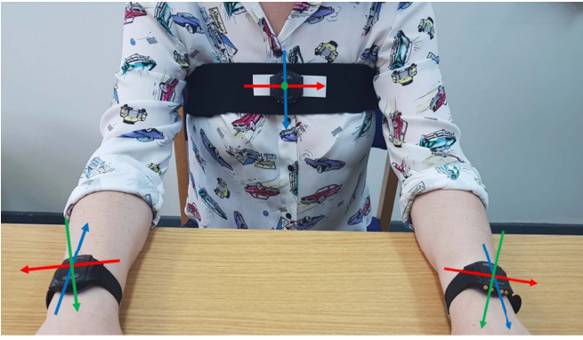
Fig. 2. The placement and orientation of accelerometers on the wrists and chest of a participant. In the image, the x-axis is red, y-axis is blue and z-axis is green. The z-axis for the chest sensor (green) is pointing away from the viewer.
