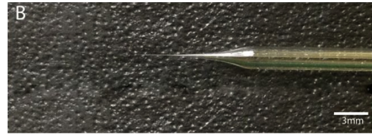
Fig. 2. The tip of the glass electrode.
