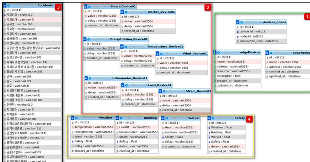
**Fig. 15.** Entity relationship diagram for the proposed construction worker safety inference system database.
