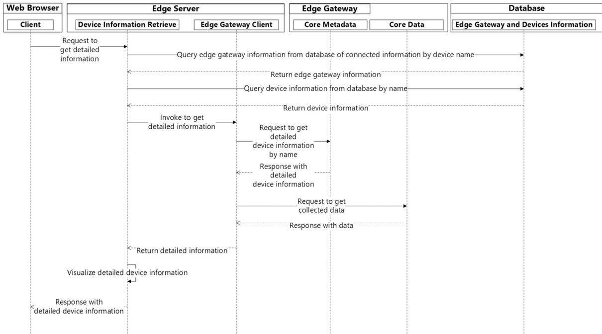
Fig. 6. Sequence diagram for detailed device information visualization.
