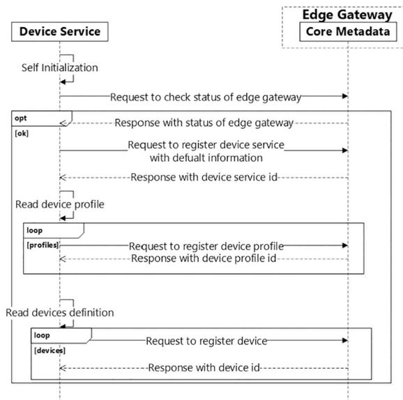
Fig. 8. Sequence diagram for device service initialization.
