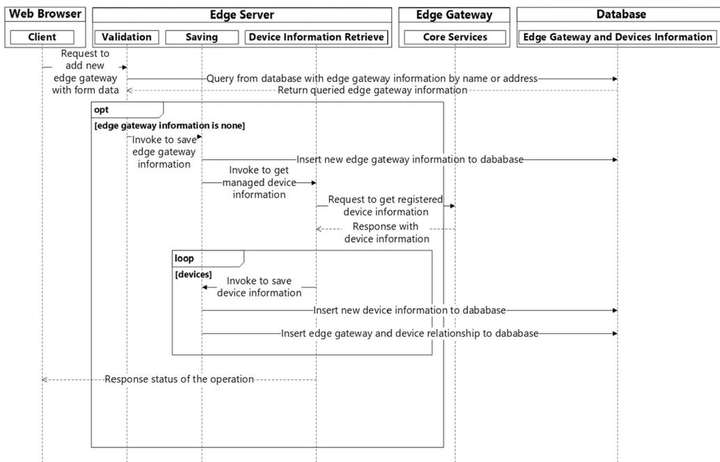
Fig. 5. Sequence diagram for edge gateway registration to the safety inference system.
