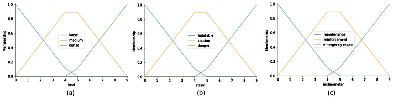
Fig. 11. Fuzzy logic fuzzification for building: (a) Fuzzy sets for load, (b) Fuzzy sets for strain, (c) Fuzzy sets for inclinometer.
