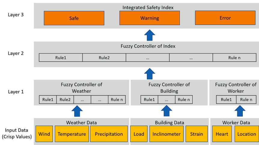
Fig. 10. Layered architecture of multi-layer rule-based modelling for worker safety index.
