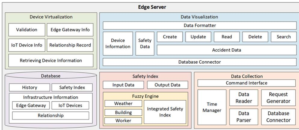
Fig. 4. Edge server architecture for device virtualization, monitoring and data visualization.
