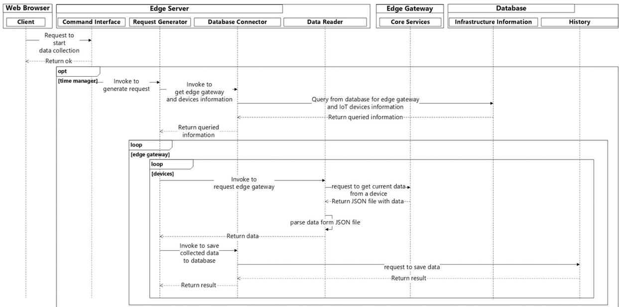
Fig. 7. Sequence diagram for data collection from simulated IoT devices.
