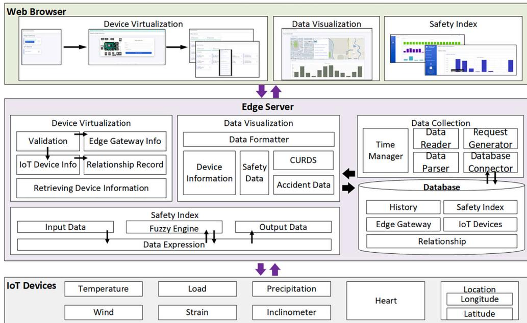
Fig. 16. Implementation configuration for worker safety inference system.
