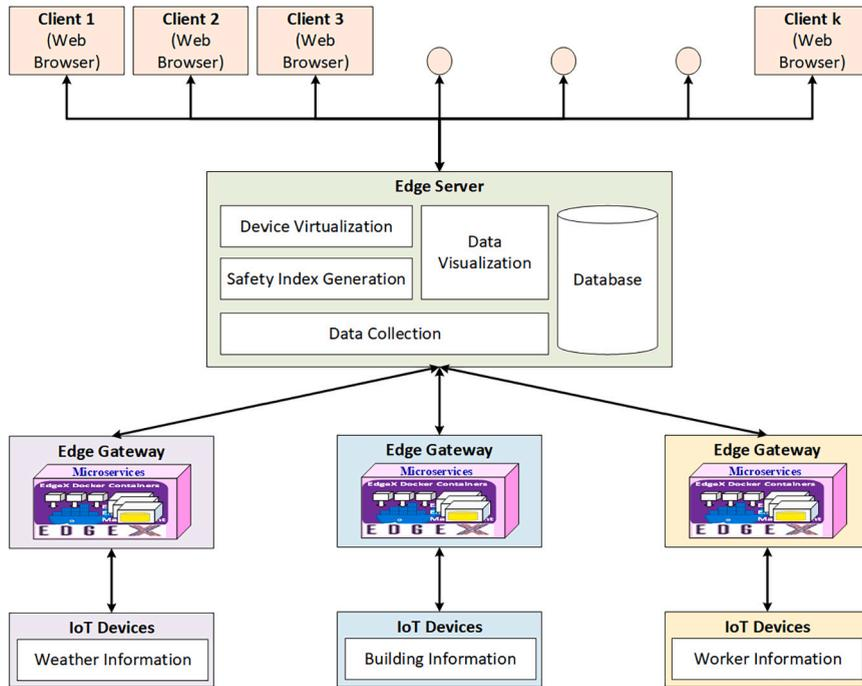
Fig. 1. Proposed conceptual architecture for worker safety inference in outdoor construction AIoT environment.
