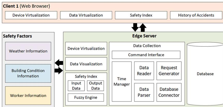
Fig. 2. Block diagram of construction worker safety inference system.
