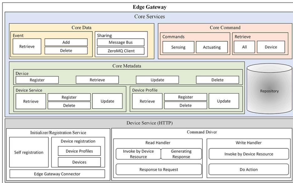
Fig. 3. Edge gateway functional block diagram for data collection.
