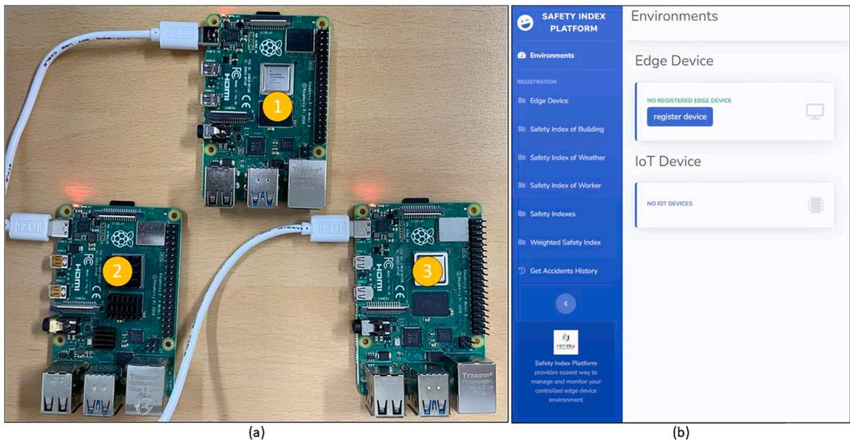
Fig. 20. (a) Edge gateway execution testbed environment. (b) Worker safety inference system main display page.
