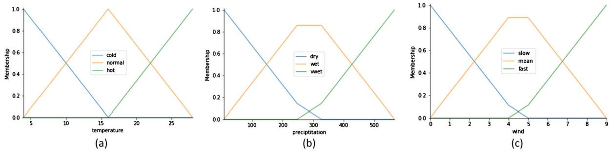
Fig. 12. Fuzzy logic fuzzification for weather: (a) Fuzzy sets for temperature, (b) Fuzzy sets for precipitation, (c) Fuzzy sets for wind.
