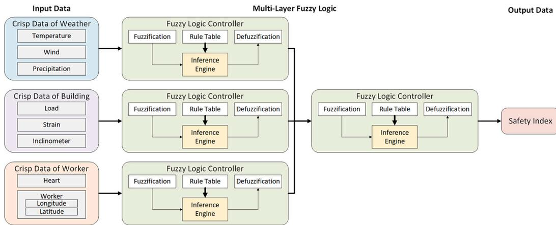
Fig. 9. Multi-layer fuzzy logic architecture for worker safety inference engine.
