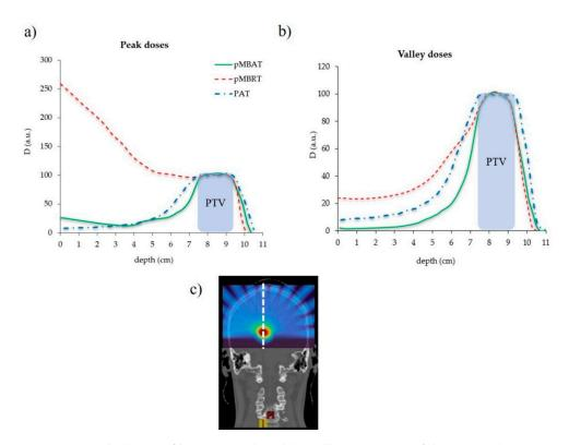
**Figure 4.** Depth dose profiles at (**a**) peak and (**b**) valleys positions of the standard pMBRT (single array), PAT and pMBAT (multi-array) scenarios. The profile considered is represented by a dotted white line in (**c**). Doses are normalized to the maximum dose at peak and valleys, respectively.
