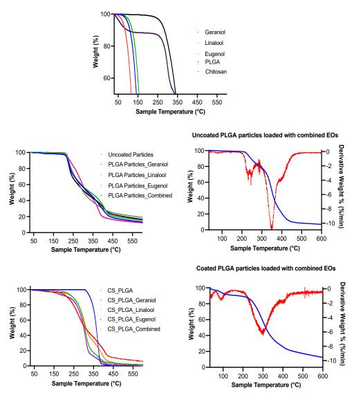
**Figure 6.** Thermogram of chemicals used to prepare the particles, EO components, plain and loaded PLGA particles (uncoated or coated), and the corresponding derivatives; thermogravimetry (DTG) analysis on the right side.
