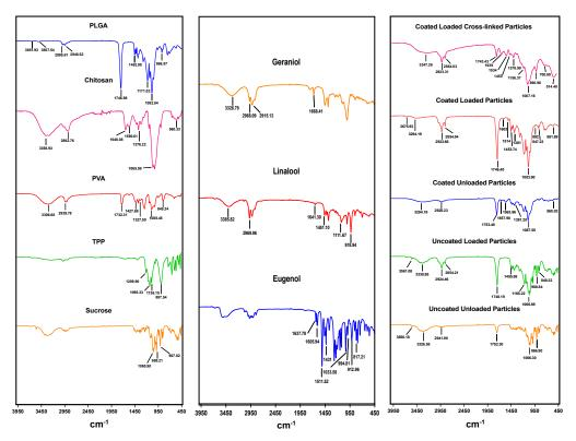
**Figure 5.** Fourier transform-infrared spectra of pure chemicals used to prepare the particles, EO components, plain and loaded PLGA particles (uncoated or chitosan coated), and crosslinked particles prepared in the study.
