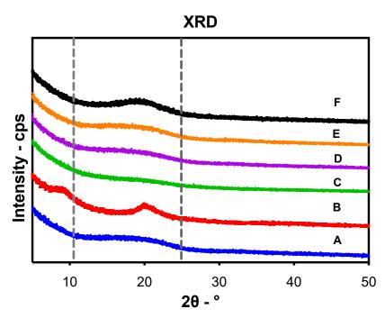
**Figure 7.** Powder X-ray diffractograms of **(A)** PLGA, **(B)** chitosan, **(C)** uncoated PLGA particles, **(D)** uncoated PLGA particles loaded with combined oils, **(E)** CS-PLGA particles, and **(F)** CS-PLGA particles loaded with combined EO components.
