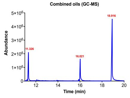
**Figure 3.** Chromatogram of the combined EO components encapsulated in the prepared particles with retention times 11.326, 16.021, and 18.916 for linalool, geraniol, and eugenol, respectively.
