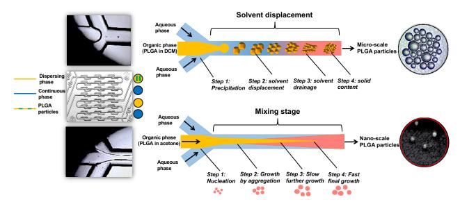
**Figure 1.** A schematic diagram of the microfluidic chip used (hydrophilic micromixer) and the process of the formulation of micro and nanoparticles.
