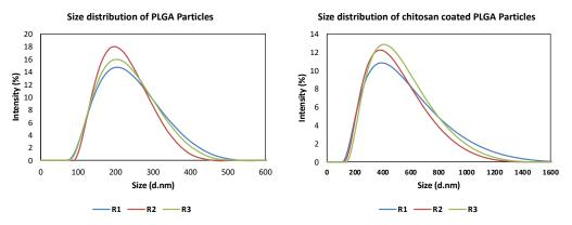
**Figure 2.** Size distribution by intensity of the uncoated PLGA and CS-PLGA particles. R1, R2, and R3 denote the replicates R1, R2, and R3, respectively.
