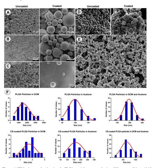
**Figure 4.** SEM micrographs showing the PLGA particles prepared using different conditions. (**A**) Uncoated and CS-PLGA particles prepared by conventional method. (**B**) Uncoated and CS-PLGA particles prepared by microfluidics using DCM as EO solvent. (**C**) Uncoated and CS-PLGA particles
