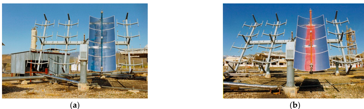
Figure 8. Former SOLARIS loop at the Plataforma Solar de Almería (PSA) near Tabernas, Spain, in 1992. (a) Used for a methylene blue and (b) rose bengal-sensitized photooxygenation.
