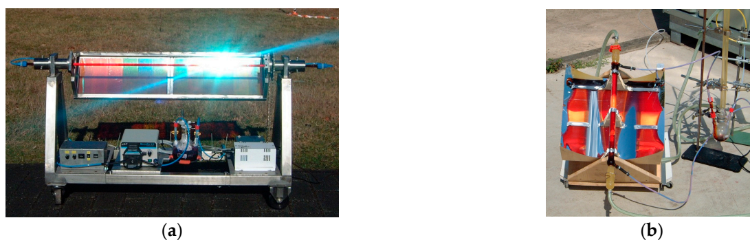
Figure 9. Laboratory-scale parabolic trough concentrators at the German Aerospace Center (DLR) in Cologne-Porz, Germany. (a) Horizontal trough reactor equipped with holographic mirrors (the reflected green light can be clearly seen), 2003. (b) Vertical trough reactor based on a Liebig condenser, 2003 (taken from [115]).
