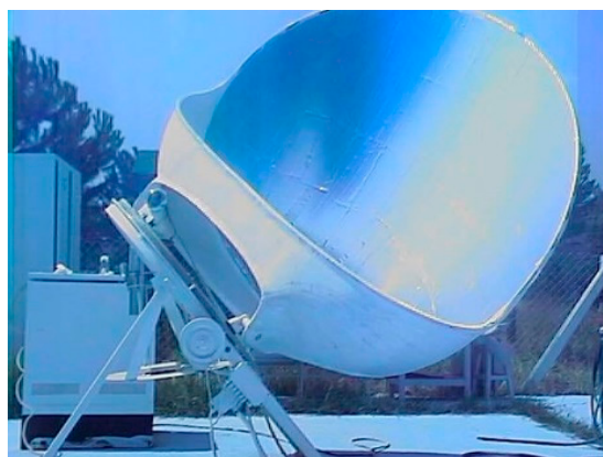
Figure 3. Parabolic dish solar concentrator (HTC Solar Research GmbH, Germany) at Ege University in Izmir, Turkey, around 2001 (taken from [83]).
