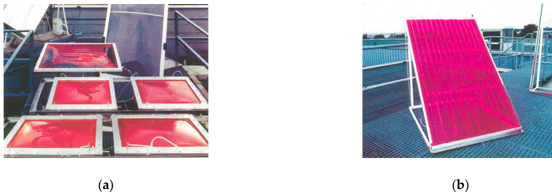
Figure 4. Examples of flatbed reactors developed by Prof Martin Demuth at the former Max Planck Institute for Radiation Chemistry in Mülheim/Ruhr, Germany, between 1998–2000 (taken from [90]). (a) Horizontal ULCR-1T reactors. (b) Tilted ULCR-4P reactors.
