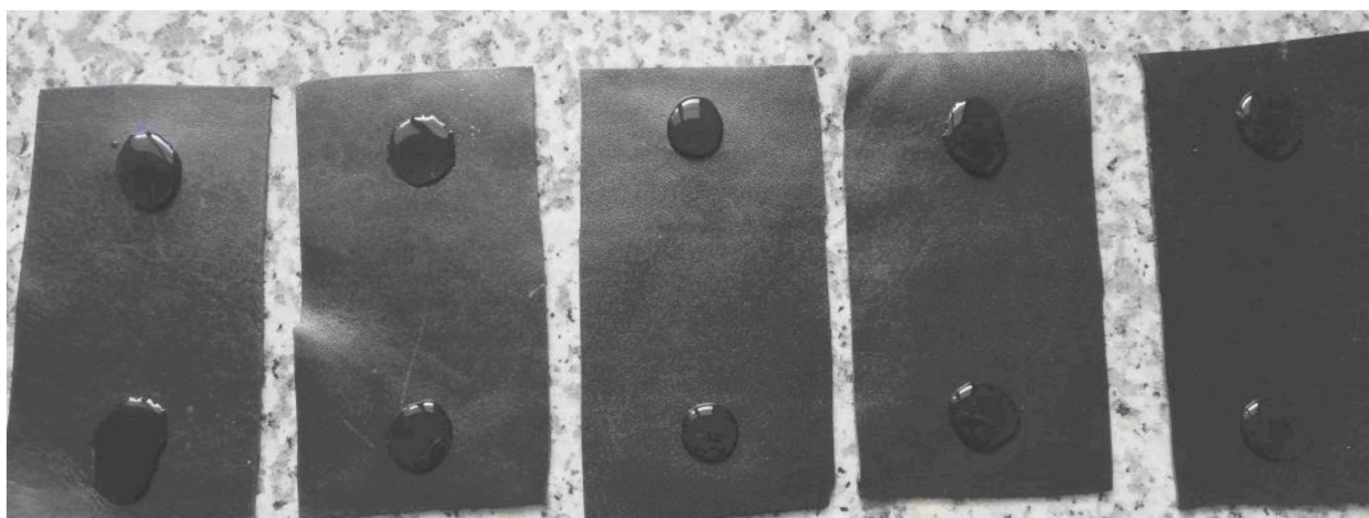
Figure 6. The images of the leather specimens during water spotting test after 30 min. (Samples from left to right: DS 90/10, DS 80/20, DS 75/25, DS 60/40, DS 50/50).
