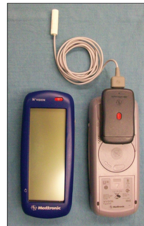
Figure 1: Front (left) and back (right) views of clinician programmer (model 8840, Medtronic, Minneapolis, MN) with external neurostimulator (model 37022, Medtronic) attached to the back of the programmer. The programmer has been updated (model 8870 version AAO Application Card, Medtronic). Also shown is the deep brain stimulation specific external neurostimulator twist-lock screening cable (model 3550-68, Medtronic) which connects the external neurostimulator to a deep brain stimulation lead. In addition to intraoperative test stimulation using the programmer, the system makes possible check of impedances specific to the deep brain stimulation lead and thus the integrity of the lead. Deep brain stimulation specific external neurostimulator screening cable with alligator clips (not shown) rather than twist-lock may be used.
