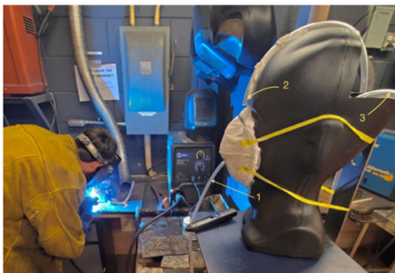
Figure 2. Respirator testing setup with numbered probes.
