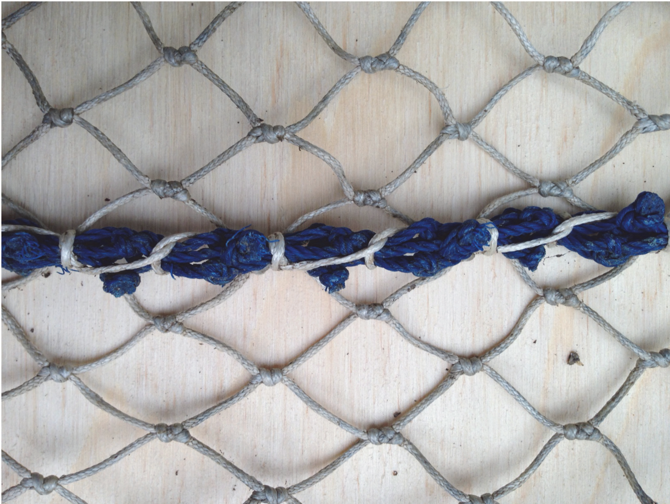
Fig 4. Stretched netting sewn down the centre line with a hanging ratio of 0.707
