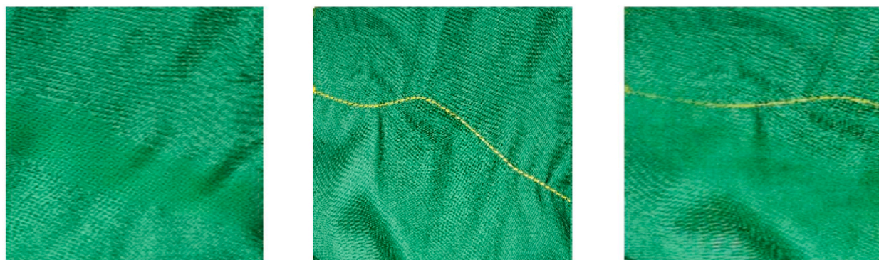
Fig. 13. Generated image of unbalanced stitch using pix2pix GAN.
