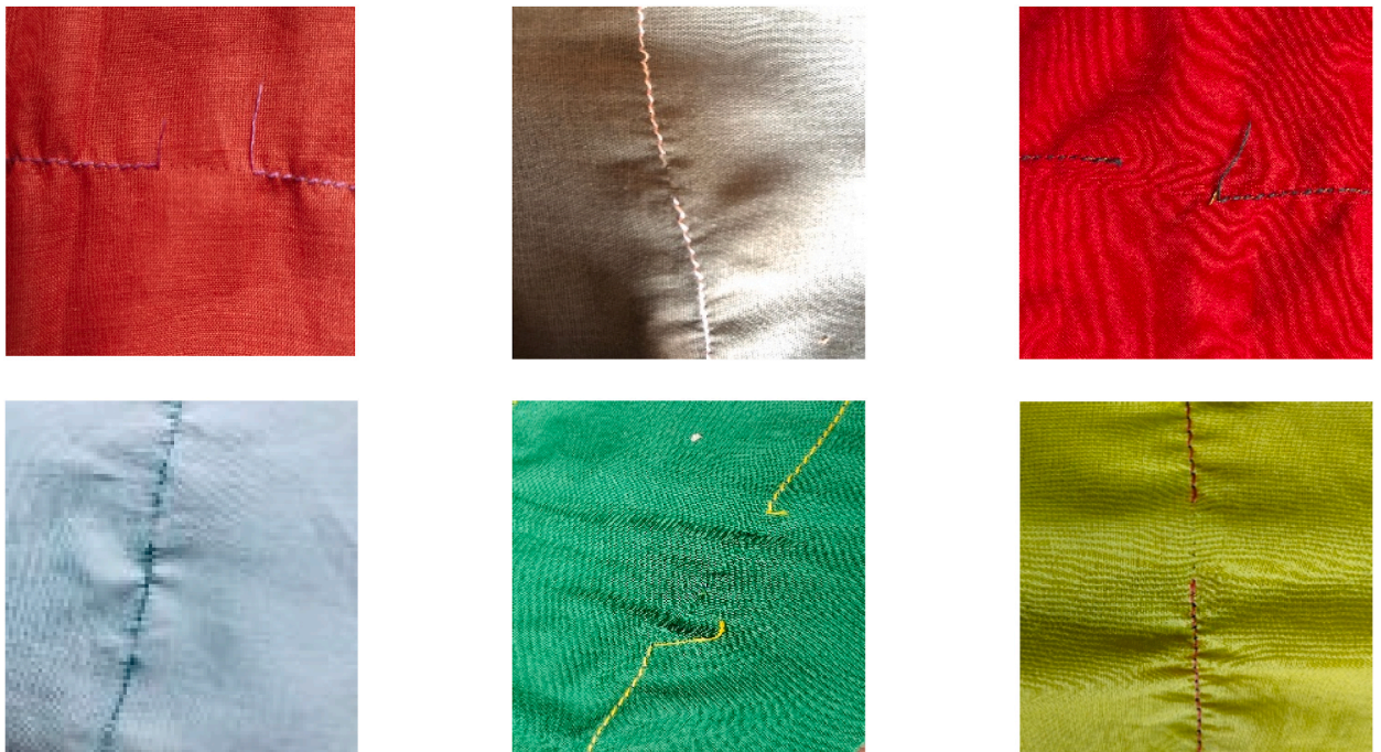
Fig. 20. Generated images of broken stitches defect.
