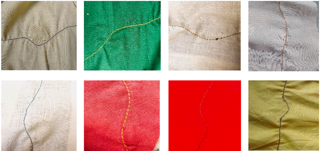
Fig. 16. Original images of unbalanced stitching defect.
