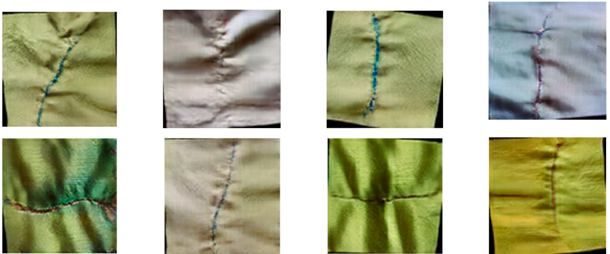
Fig. 19. Synthetic images of puckering seam defects.
