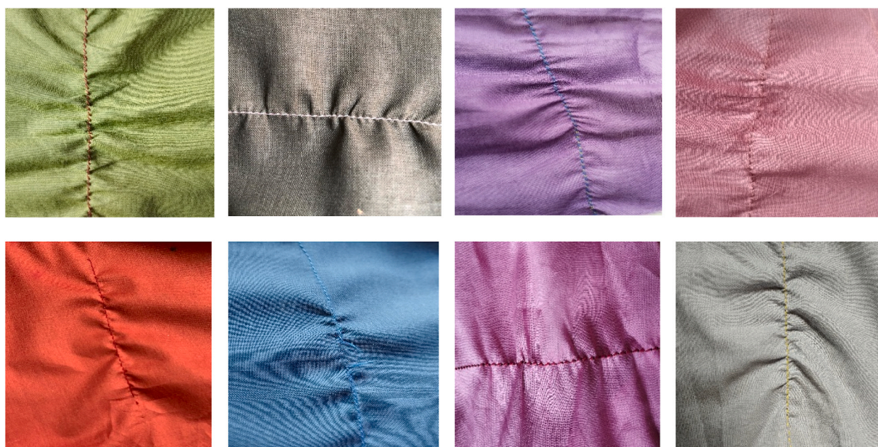
Fig. 18. Original images of seam puckering defects.
