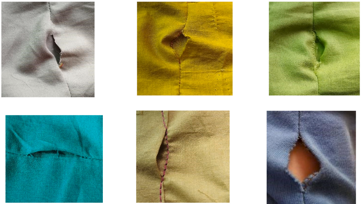
Fig. 22. Original images of open seam defect.
